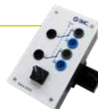
PN4034 - Emergency stop knob (electrical)
